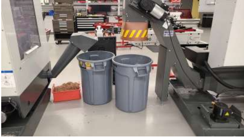
Metal Chips/Shavings Disposal
